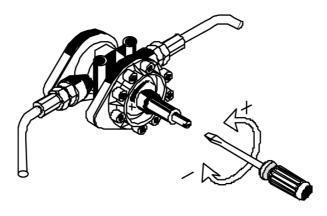
Do not adjust more than 1/4 turn at a time. The result of the adjustment can be seen on the tableware after the 5th wash.
